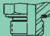
Form PEFLEX: Sealing by means of a profiled elastomer ring recessed into the fitting body. Female thread is parallel.
