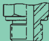
DIN 3852 Form B: Sealing by means of a sealing "shoulder."
