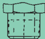
DIN 3852 Form C: Sealing by means of tapered thread. Female thread must be tapered to achieve rated operating pressure.
