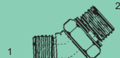
BPP-OFS-6802-NWO - 45° (1) Male O-Ring Face Seal (SAE) (2) Male BPP Adj. O-Ring w/ Retainer Washer
