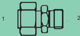
MFL-M-6510 - Str. (1) Fem. Flareless Swivel (2) Male Metric Parallel w/ Cutting Face Seal Light
